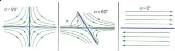
The above figure shows the particle paths of flow characteristic of three different types of deformation. From left to right they are:
