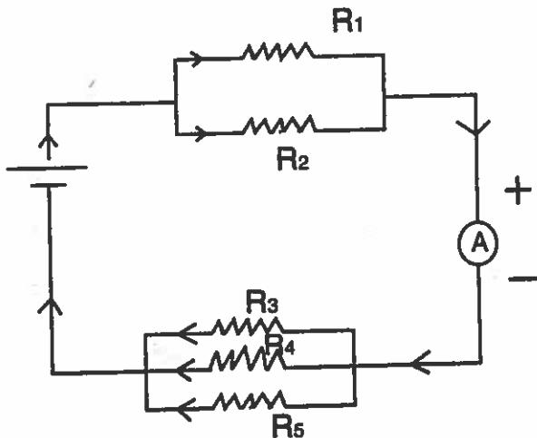
$$R_1 = 5 \Omega, R_2 = 20 \Omega$$
