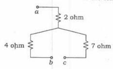
If the resistance between terminals b and c with a open is represented by  $R_A$ , the resistance between c and a with b open is represented by  $R_B$  and the resistance between a and b with c open is represented by  $R_C$ , then arrange  $R_A$ ,  $R_B$ ,  $R_C$  in descending order.
